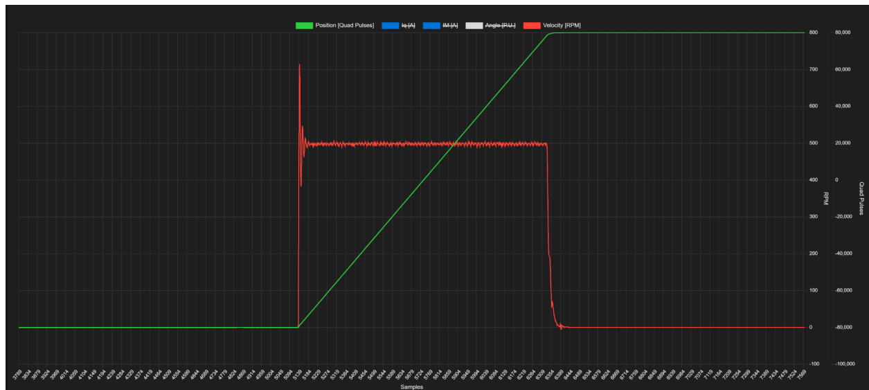
Figure 4- Position and Speed feedback shapes on step response of a PMSM in reaction to a +80,000 pulses as position set-point
